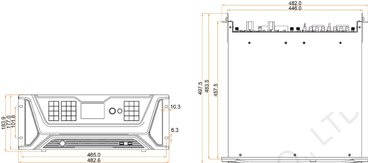
Tolerance: ±0.5 Unit: mm
